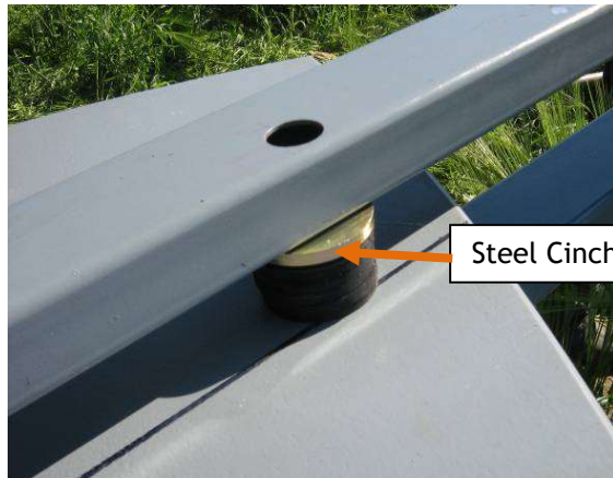
Figure 5.5 Front compliant mount assembly and washer
