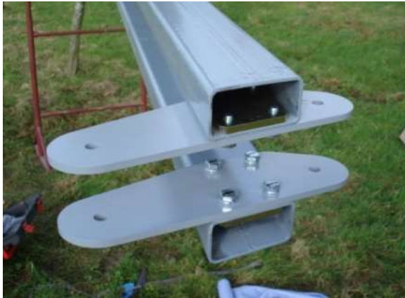
Figure 5.1 Tail Vane Support Plates
