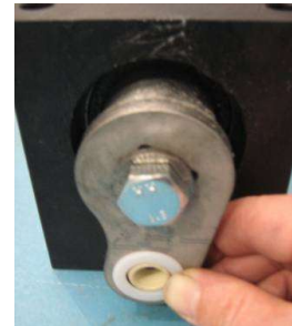
Figure 9.4 Nylon washers on pitch lever
