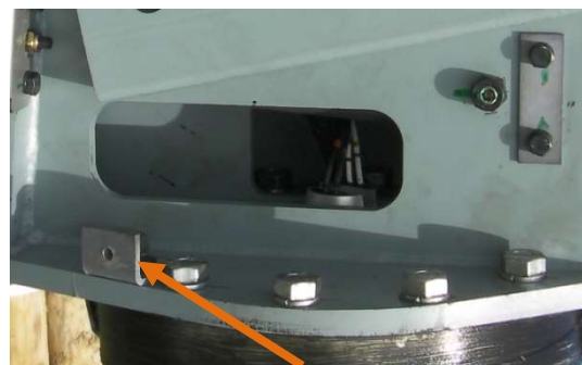
Figure 14.3 Rear Cover Yaw Box Bracket
