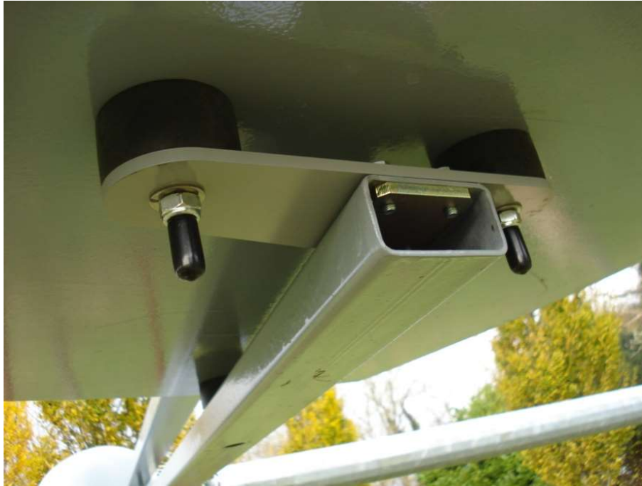
Figure 5.7 Completed Tail Vane assembly with Protective Caps fitted
