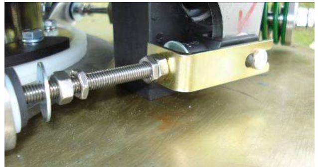
Figure 10.7 Clevis anti rotation clip nut and locknut tightened
