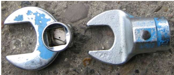
Figure 3.2 Crows foot fitting and spigot type fitting for use with a torque handle
